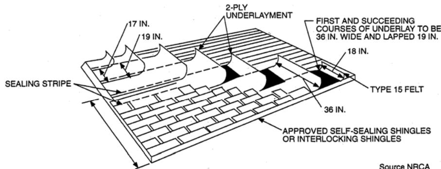
**NOTE:** In areas where average daily temperature in January is 25°F or less, felt plies of underlayment should be cemented up from eaves far enough to overlie a point 24 in. inside the inside wall line of the building.
