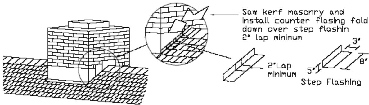
**Other flashing.** Flashing against a vertical front wall, as well as soil stack, vent pipe, and chimney flashing, shall be applied according to asphalt shingle manufacturer's printed instructions.
