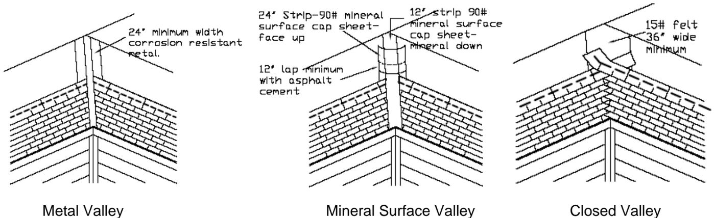
1. For open valley (valley lining exposed) lined with metal, the valley lining shall be at least 24 inches wide and of any of the corrosion-resistant metals.
