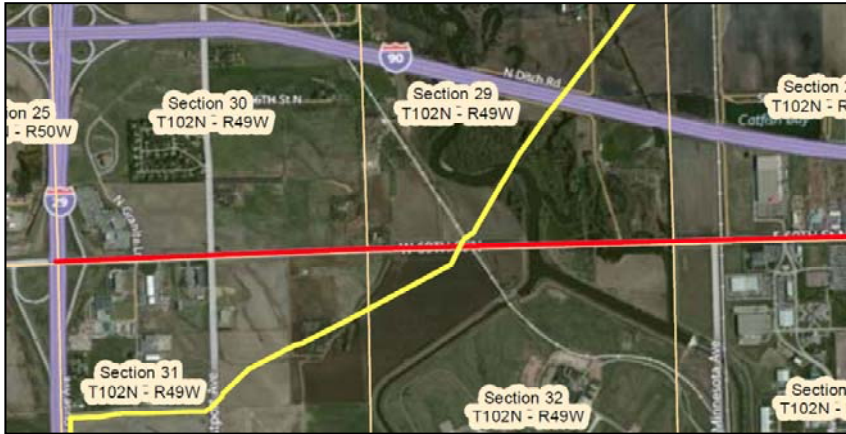
Segment 2 Utility Maps provided by Magellan indicating a large gas main crossing of 60 th Street North near the BNSF rail crossing
