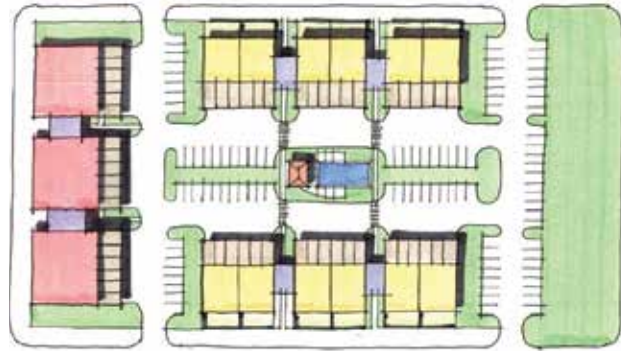
Diagram of a multifamily project with interior parking and buildings along the street frontages. Garages are incorporated into the rear facades of buildings.
