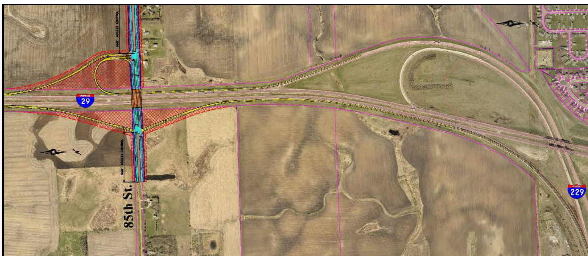
Figure 2-5: IJR Folded Diamond Interchange (Previously Dismissed)
