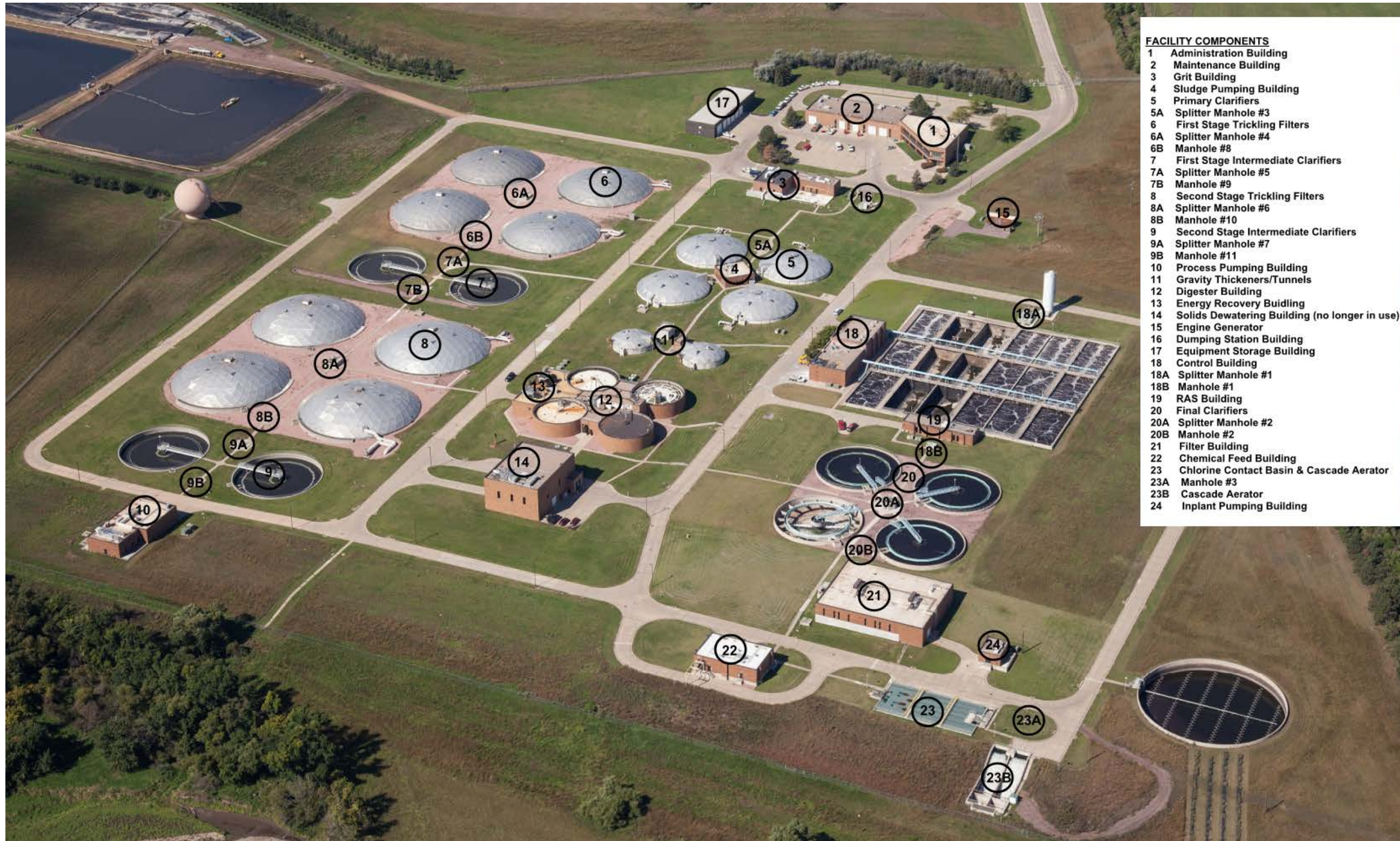
Figure 1.2 Water Reclamation Facility Process Components
