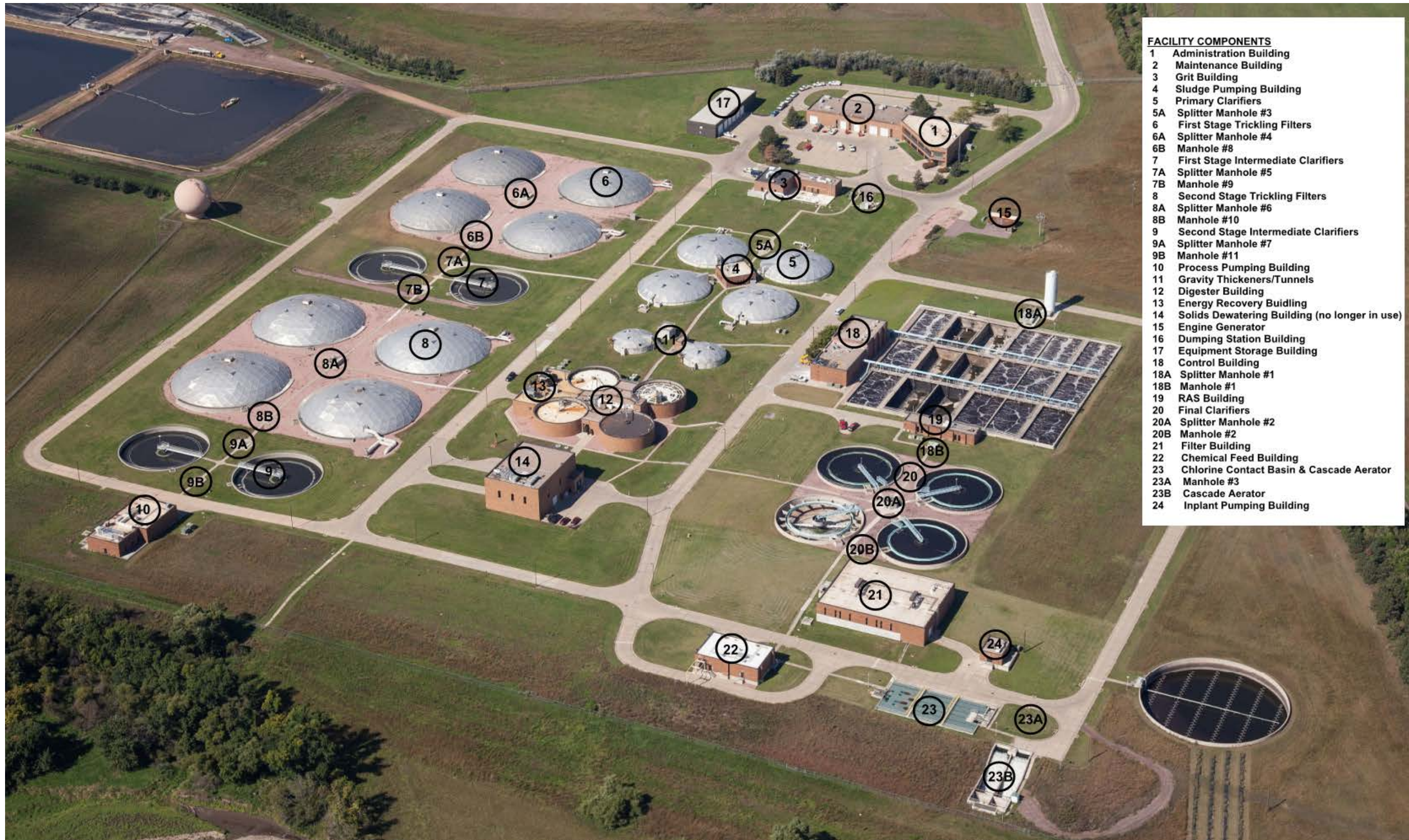
Figure 3.7 Water Reclamation Facility Process Components
