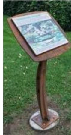
Pedestals constructed of quarter-inch corten steel display images and information at a comfortable height for visitors to read.
