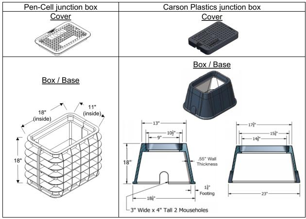
Surface Mounted Junction Box: Surface mounted junction boxes shall be used with tunnel and under bridge luminaires.
